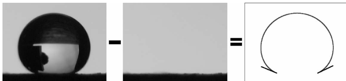
Figure 1. Extraction of the drop contour and contact angles.
